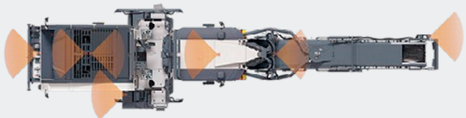
Optional camera system comprising up to seven cameras: area in front of the machine / front track units / front rotor plate / rear rotor plate / left side of the machine towards the front / paving screed / loading situation
