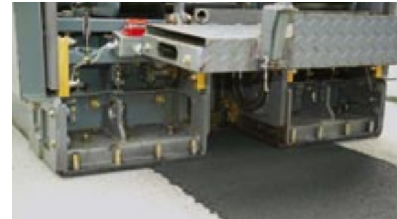
System for paving width reduction allows minimum width of 20 in.
