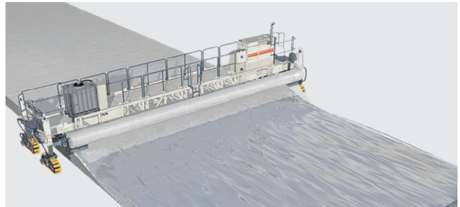
Film unroller for effective protection of the concrete in case of rain.
