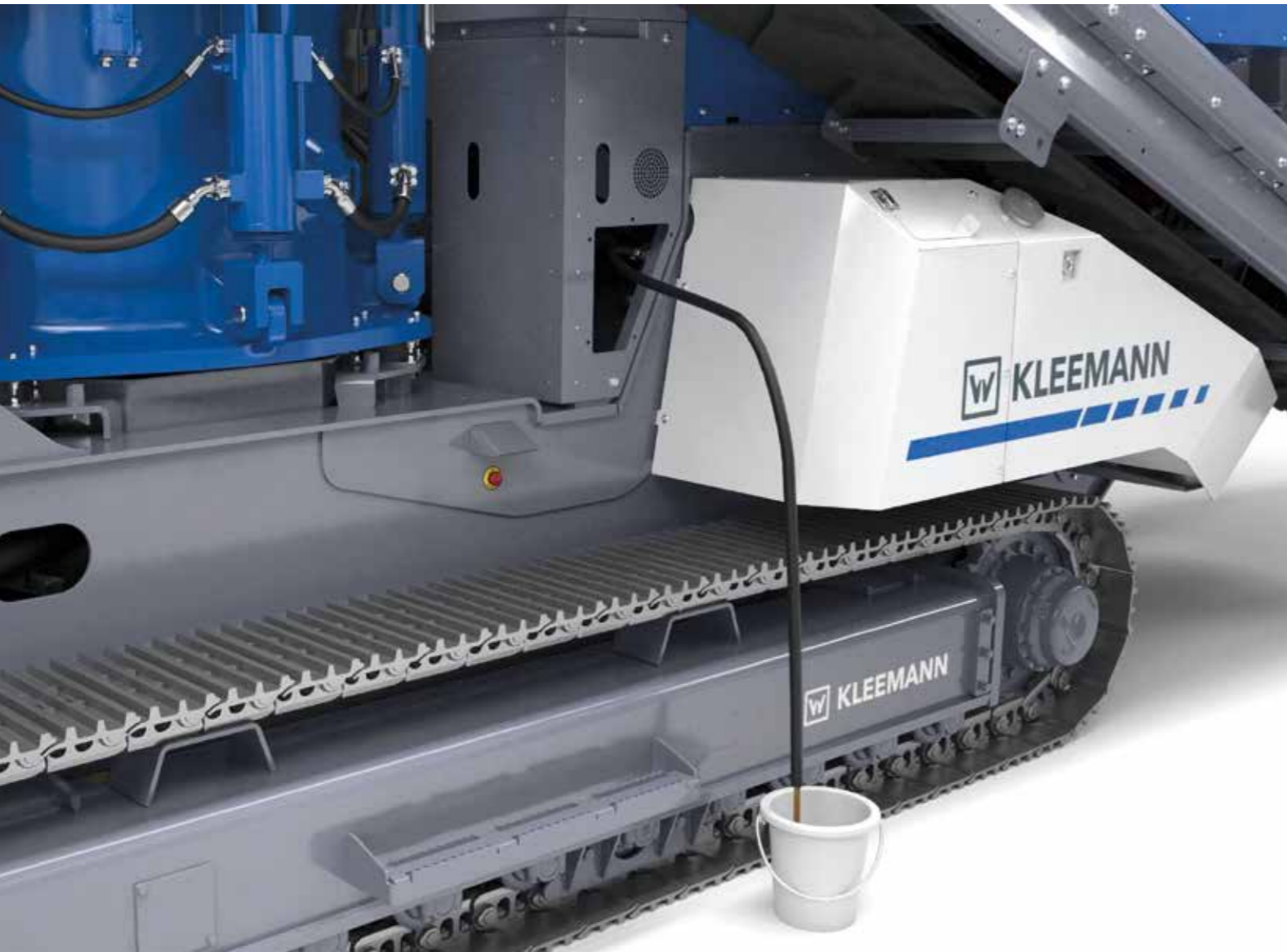
Central drain point
